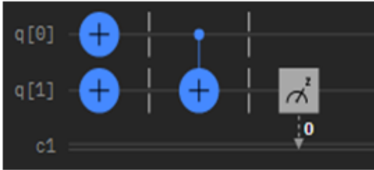
Fig. 1: Circuit diagram of Q-XOR
