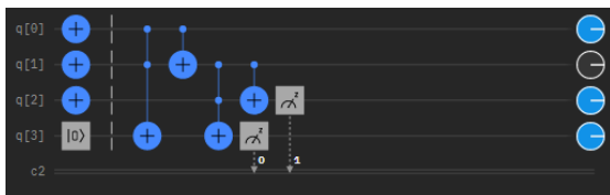
Fig. 8: Circuit diagram of q-Adder for SHA-256
