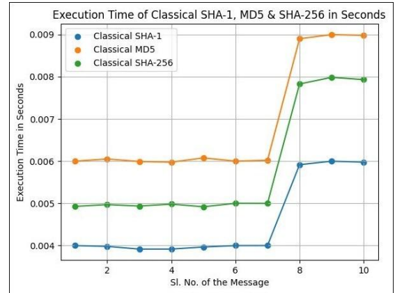
Fig. 16: Execution time of cSHA-1, cMD5 and cSHA-256 for the same inputs
