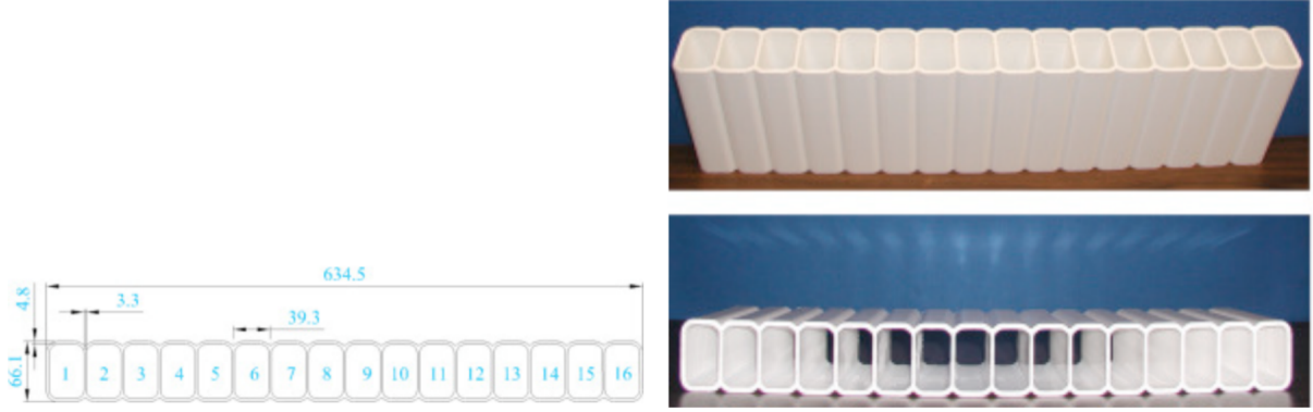
Figure 2.6: PVC extrusion modules used in the NOvA detectors. Each extrusion consists of 16 individual rectangular cells formed from rigid PVC, with approximate transverse dimensions of 3.9 \times 6.6 \text{ cm}^2 per cell. The left panel shows the technical drawing with dimensions in millimeters, while the right panels display photographs of the fabricated extrusion. These extrusions are assembled into planes, with cells filled with liquid scintillator and read out by wavelength-shifting fibers coupled to APDs.
