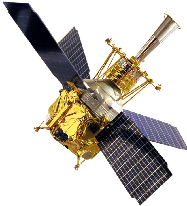
Figure 11. Spacecraft. The 5 m long 1.6 m diameter Spacecraft has four tilted solar arrays oriented to provide optimum mean power through the year, two tilted clockwise and two counterclockwise to balance torques from residual air and solar radiation pressure.
