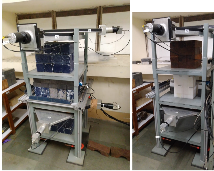
FIGURE 3.9: The configuration for the measurement of neutron production from stopping muons, in the MINT setup for Pb (left panel) and Fe (right panel).
