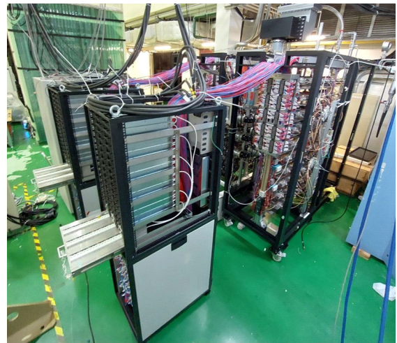
Figure 1: The 80 kW solid-state amplifier with two separate power supply racks.
