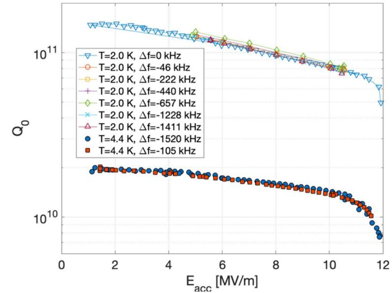
Little change in the coated cavity performance after tuning up to 1400 kHz at cryogenic temperatures
