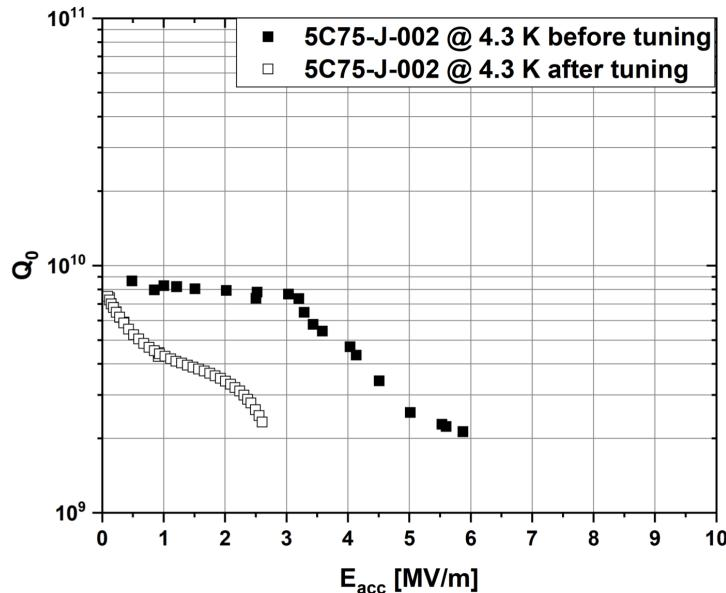
Strong degradation in the coated cavity performance after room temperature tuning for 200 kHz
