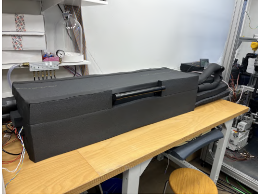
Figure A.2: Left: picture of the closed module cooling box in the laboratory. The connection of the cooling structure inside the box to the CO 2 cooling system is made from the right side of the box. The chiller that actively cools the module cooling box is connected on the left side. It is not visible in this picture. Right: picture of the CO 2 cooling system in the laboratory. The main tubing as well as the CO 2 pump, the flow meter, the pressure sensors et cetera are located in the ITEM rack on the left. The two big Huber chillers that are used to control the temperature of the accumulator vessel and the heat exchanger that is installed before the CO 2 pump can be seen on the right next to the rack.
