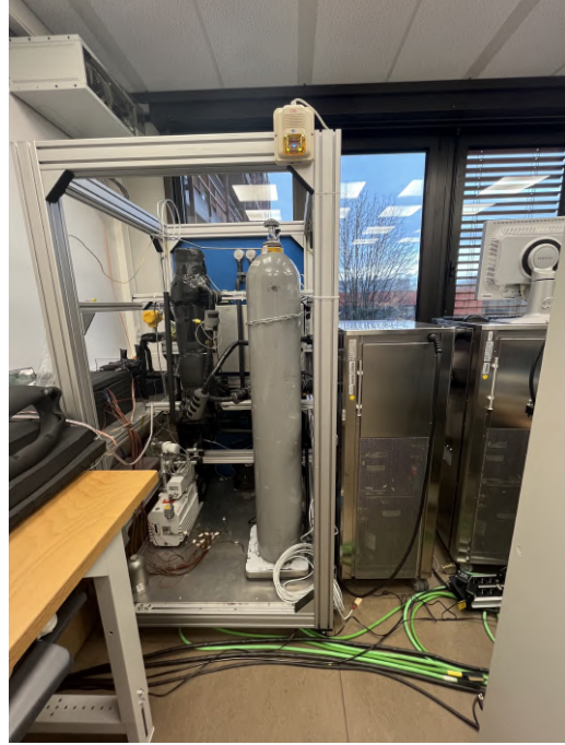
Figure A.2: Left: picture of the closed module cooling box in the laboratory. The connection of the cooling structure inside the box to the CO 2 cooling system is made from the right side of the box. The chiller that actively cools the module cooling box is connected on the left side. It is not visible in this picture. Right: picture of the CO 2 cooling system in the laboratory. The main tubing as well as the CO 2 pump, the flow meter, the pressure sensors et cetera are located in the ITEM rack on the left. The two big Huber chillers that are used to control the temperature of the accumulator vessel and the heat exchanger that is installed before the CO 2 pump can be seen on the right next to the rack.
