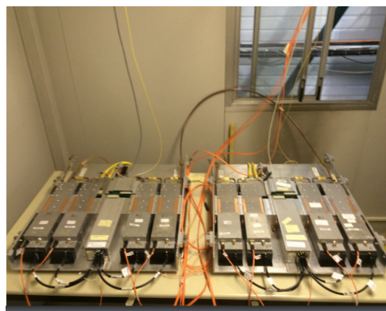
Figure 4.11: Test stand set-up at CMS detector site for SiPMs testing.
