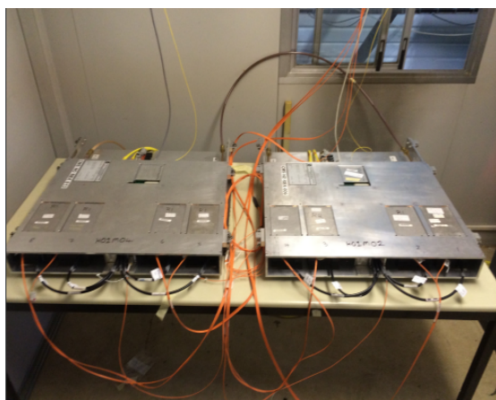
Figure 4.11: Test stand set-up at CMS detector site for SiPMs testing.
