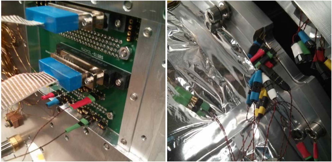
Figure 27: The 60 K cold break out board. The left picture shows the side facing the 4 K stage. Signals to the colder stages continue on MDM wire harnesses while the 60 K signals are broken out on SIP connectors. The right image shows the connectors bridging the 60 K shield. When the shield is removed for service these connections have to be broken. To facilitate easy reconnection the connectors are color coded and the polarity is marked.
