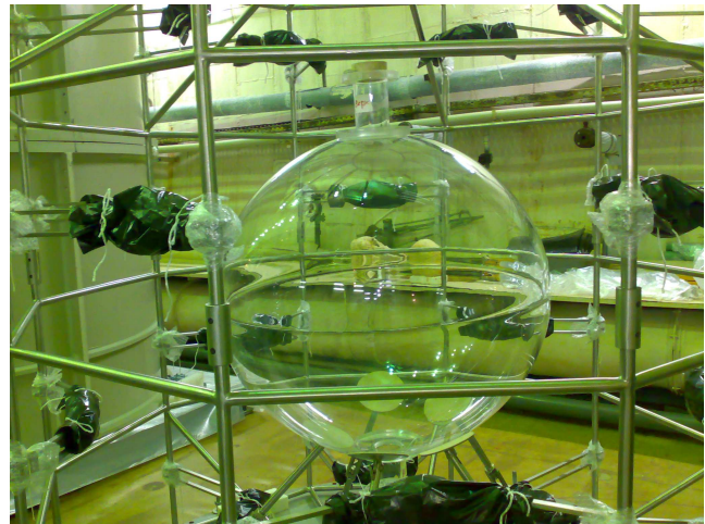
Figure 2. The acrylic sphere with stainless steel supporting structure.
