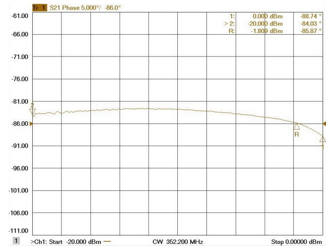
Figure 3: Phase variations within 20dB input dynamic range for 2kW amplifier (5°/div).
