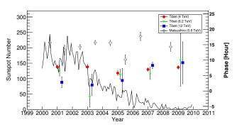
**Figure 2:** The phases of the "additional" anisotropy observed by the Tibet experiment at 4.0 TeV (red circles), 6.2 TeV (green pentagrams) and 12 TeV (blue squares), in comparison with the Matsushiro experiment at 0.6 TeV (gray crosses). The errors are all statistical only. The yearly mean phase observed by Matsushiro in 2007 is omitted in order to exclude large fluctuation due to the insignificant anisotropy. The gray line indicates the monthly mean sunspot number.
