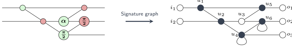
Figure 3.3: A graph-like ZX-diagram \mathcal{D} and its associated signature graph \mathcal{G}_{\mathcal{D}} . The input vertices are \mathcal{I} = \{i_1, i_2\} and the output vertices are \mathcal{O} = \{o_1, o_2, o_3\} . The set of vertices \mathcal{P} associated with spiders whose phases are multiples of \pi/2 are shown in black.
