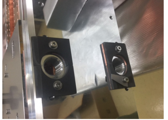
FIG. 11. Two pairs of ferrite dampers installed on top of the in vacuum girder of the SPEAR3 BL17 ID. (Courtesy of Neomax Engineering Co.)
