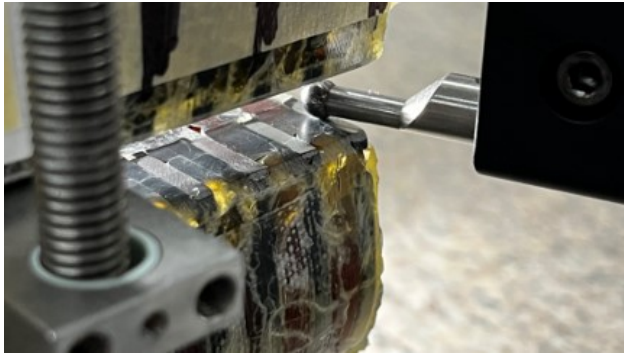
Figure 3: Linear height gauge probe during the magnetic gap measurement.
