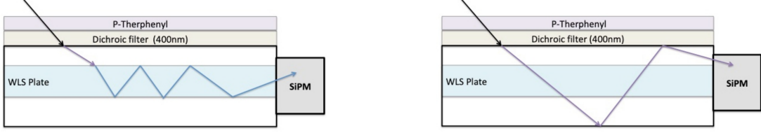
Figure 3.22: Illustration of the operational principle of an X-ARAPUCA photon detector showing the two mechanisms by which incident photons can be trapped. Figure from Reference [216].
