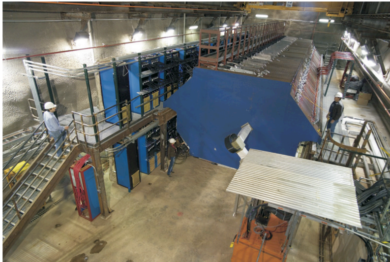
Figure 3.14: Photograph of the MINOS-ND in the MINOS near detector hall at Fermilab prior to ArgoNeuT’s installation. The squashed-hexagonal shaped steel planes that make up the detector can be seen, along with the magnetic coil entering the upstream face. Image from Reference [238].
