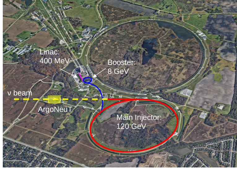
Figure 4.1: Aerial view of the NuMI neutrino beam at the Fermi National Accelerator Laboratory. The approximate locations of the Linac, the Booster and Main Injector synchrotrons and the ArgoNeuT detector are shown. Image adapted from Reference [260].
