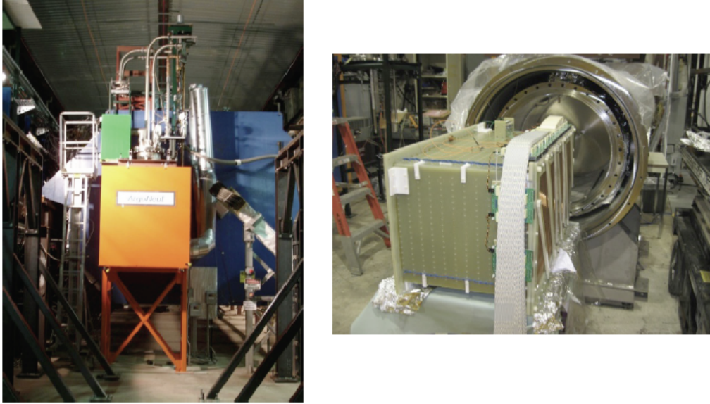
Figure 3.12: Left: photograph of the ArgoNeuT detector structure (orange box), with the MINOS-ND behind it (blue structure). Right: photograph of the ArgoNeuT TPC prior to it being inserted into the cryostat, seen behind it. Images from Reference [172].
