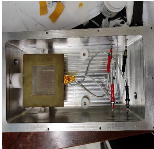
Figure 1. THGEM foil used for the experiment Figure 2. Aluminium box containing all the connections
