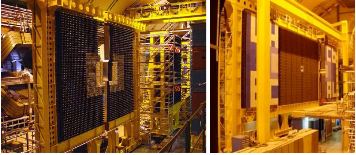
Figure 2.19: The electromagnetic calorimeter (left) and hadronic calorimeter (right) during installation of the LHCb detector at Point 8 [27].
