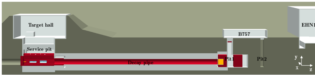
Figure 43: Side view of the CENF facility and the following experimental hall EHN1 as implemented in FLUKA. Iron is displayed in red, concrete in grey, aluminium in light blue, graphite in yellow and moraine in khaki.
