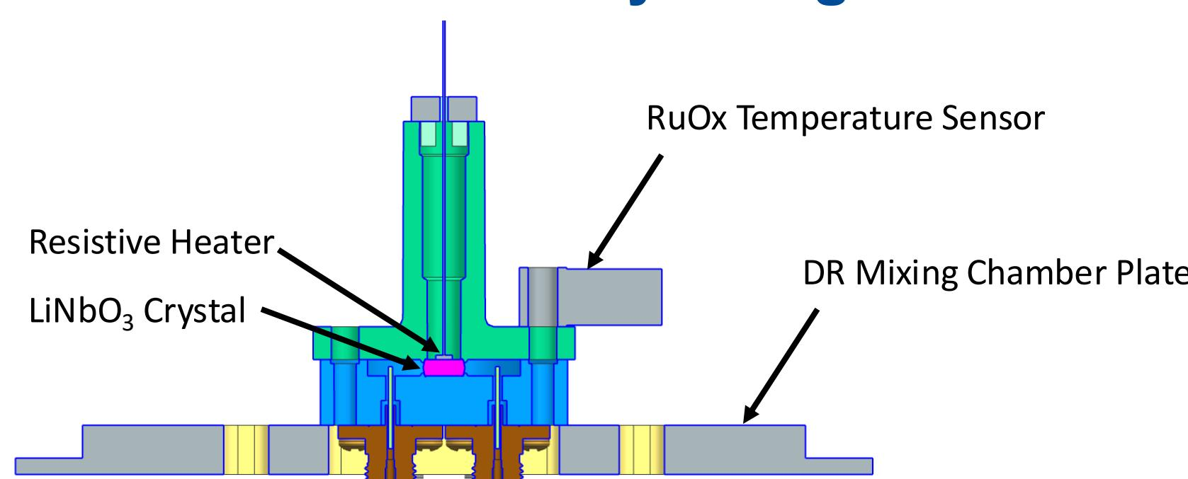
The quantum transduction cavity is mounted in a Dilution Refrigerator (DR) at mK with temperature sensors and a resistive heater epoxied to the  $\text{LiNbO}_3$  optical resonator to simulate laser pump heat loads and pumping schemes. Experiments will inform design to reduce thermal noise from laser pump.
