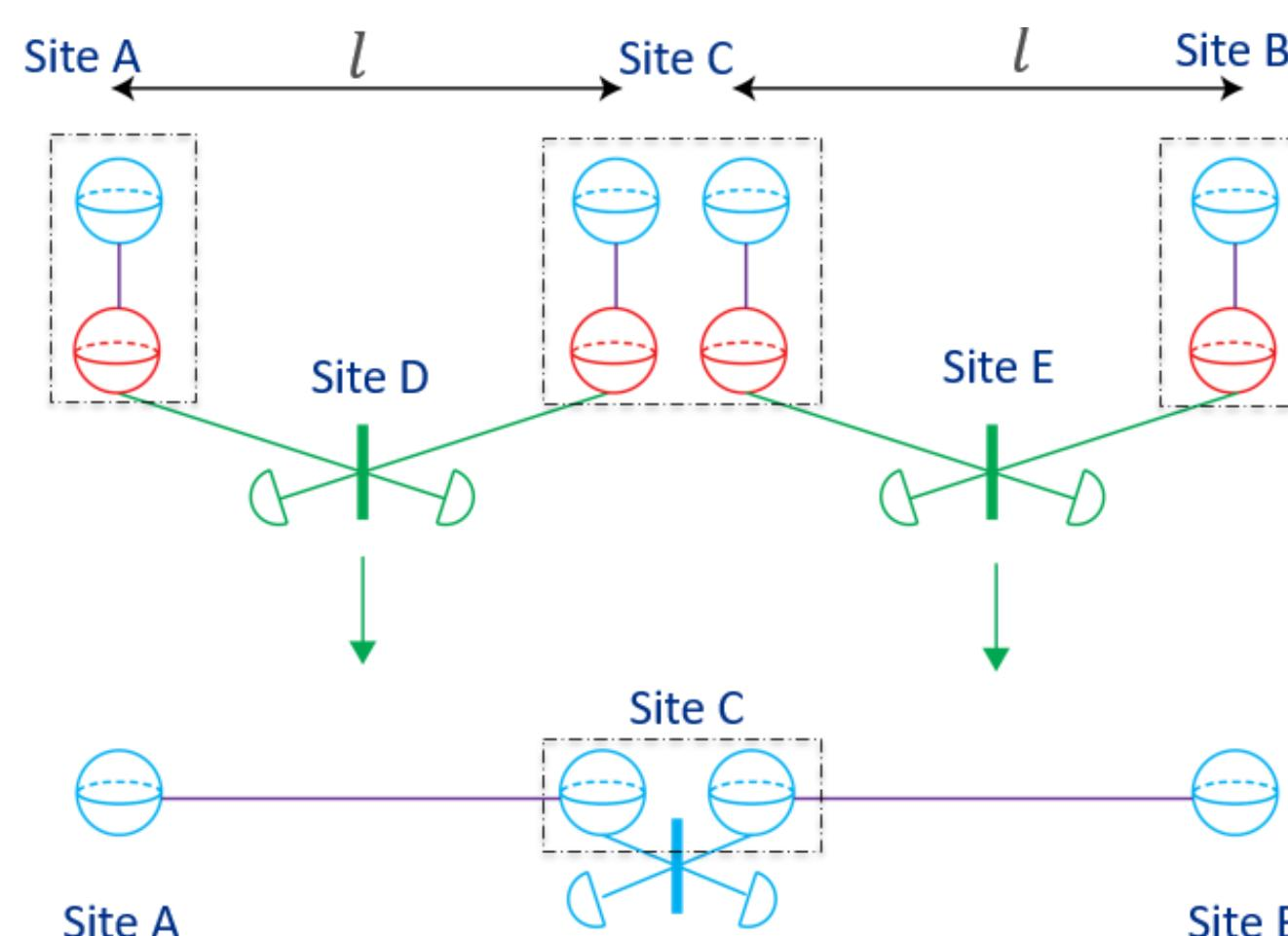
Compared to a full optical quantum repeater design, the hybrid design performs quantum swaps at site C with significantly higher efficiency than 50%.
