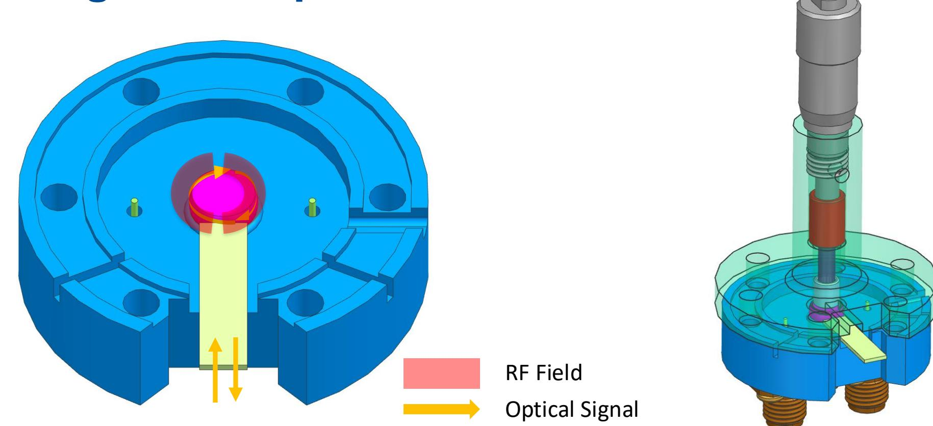
3D hybrid quantum system: a tunable SRF cavity embedded with a lithium niobate ( $\text{LiNbO}_3$ ) optical resonator. A laser pump is coupled to the  $\text{LiNbO}_3$  WGM resonator via lensed fibers and a waveguide chip coupler.
