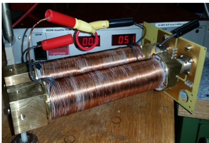
Figure 5.16: Prototype of the grid variable inductance. Two shorted coaxial line are in parallel with respect to the RF path and connected to a PCB. The latter contains the sockets for the Bias connections, the capacitors decoupling the DC from the RF paths, and the pins for the connections to other devices.
