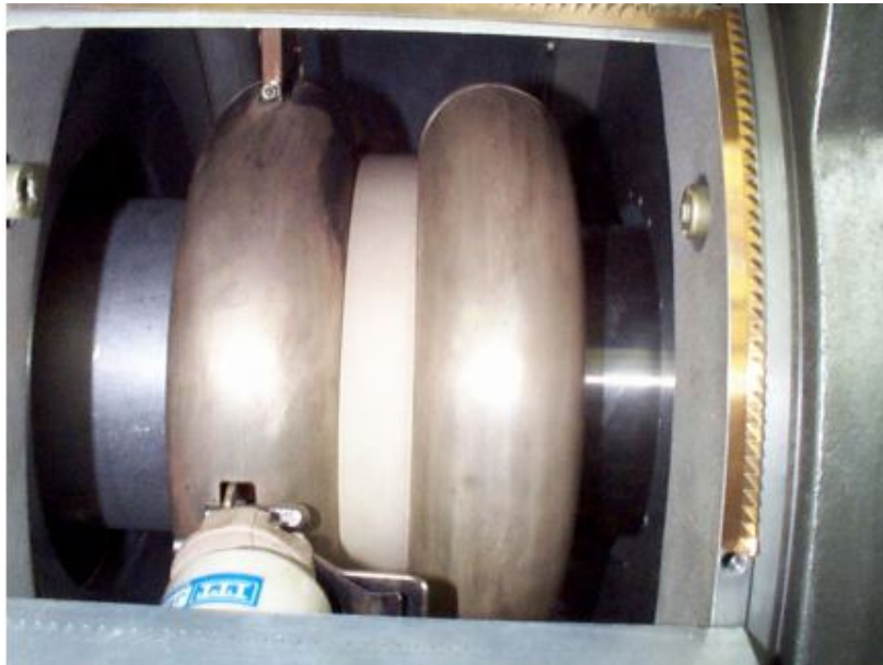
Figure 42: Gap of the 10MHz cavity.
