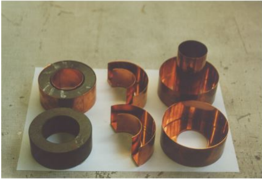
Figure 45: Pieces of the autotransformer.
