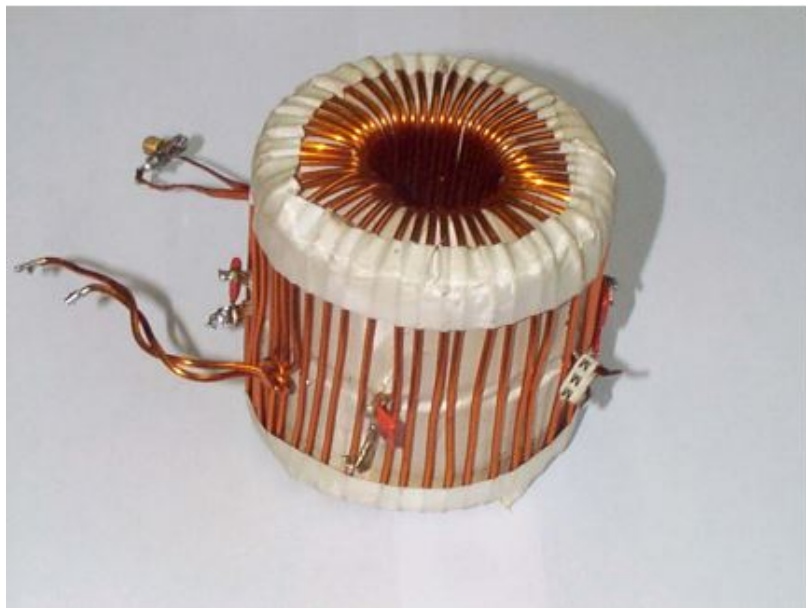
Figure 44: Old magnetically tunable autotransformer.
