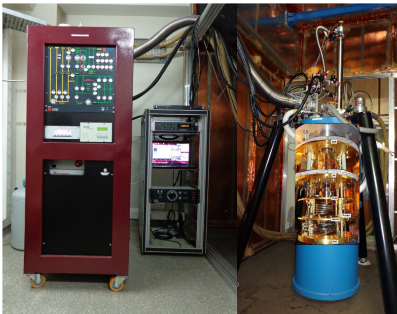
Figure 1. The CFDR-1200 set up at TIFR for Sn bolometer development
