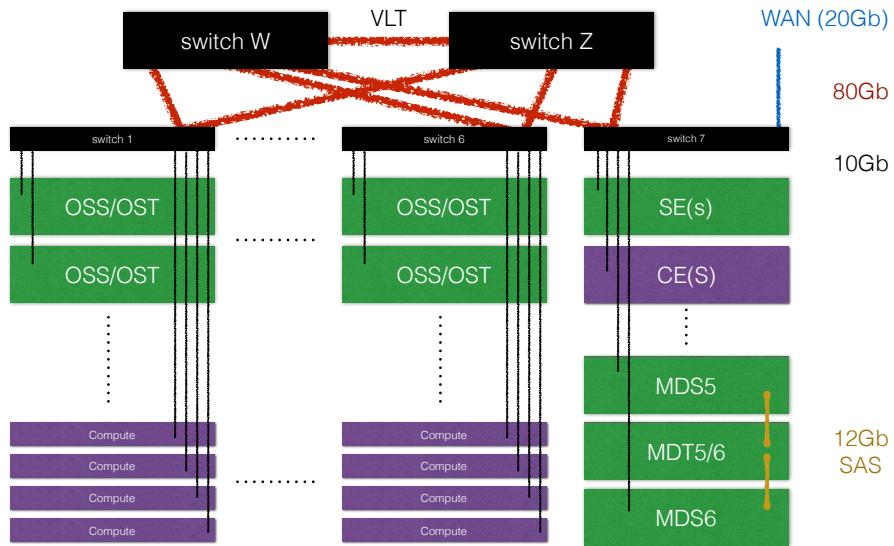
**Figure 1.** Queen Mary GridPP Cluster Layout including the StoRM Storage Element (SE) and Cream Compute element (CE)
