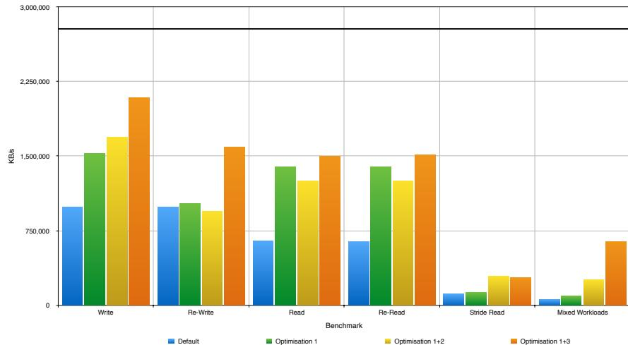
**Figure 2.** Effect of tuning on single server storage performance
