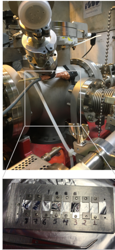
Figure A.1: Top: Collection chamber at the end of the General Low Mass beamline at ISOLDE-CERN. Bottom: Implantation matrices of Ta, C, Ni, Al, Ti mounted on an Al sample holder in 2018. Different implantation materials were tested to optimize subsequent xenon extraction.
