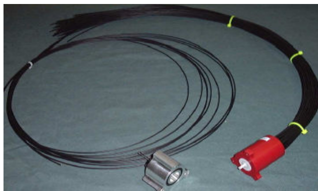
Figure 6.4: A photograph of a prototype cone and LI fibre “pigtail”. The legs of the LED can be seen poking out of the back of the cone. The snout of the pigtail connector fits into the open end of the cone.
