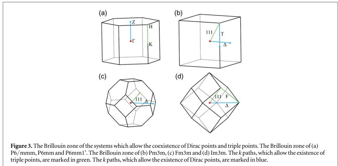
**Figure 3.** The Brillouin zone of the systems which allow the coexistence of Dirac points and triple points. The Brillouin zone of (a) P6/mmm, P6mm and P6mm1'. The Brillouin zone of (b) Pm3m, (c) Fm3m and (d) Im3m. The  $k$  paths, which allow the existence of triple points, are marked in green. The  $k$  paths, which allow the existence of Dirac points, are marked in blue.
