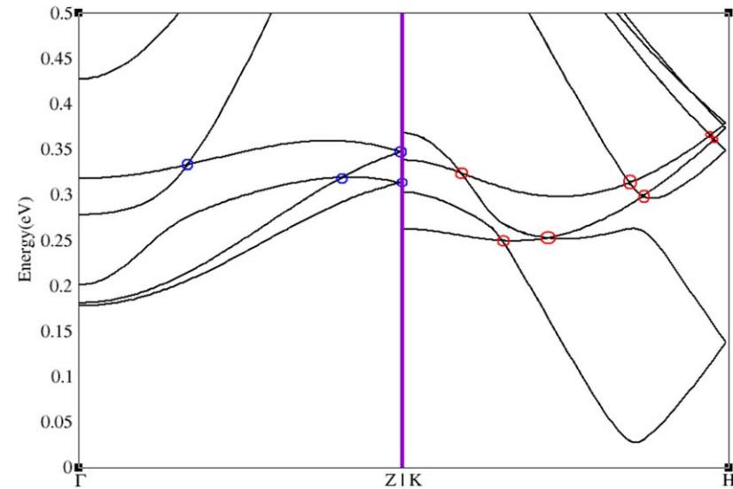
**Figure 6.** The band structure along  $\Gamma-Z$  and  $K-H$  for  $\text{As}_2\text{Ni}_5$ . The Fermi energy is set to be zero. Those Dirac points and triple points, which are in the energy range of 0.25 eV–0.37 eV, are marked in blue and red, respectively.
