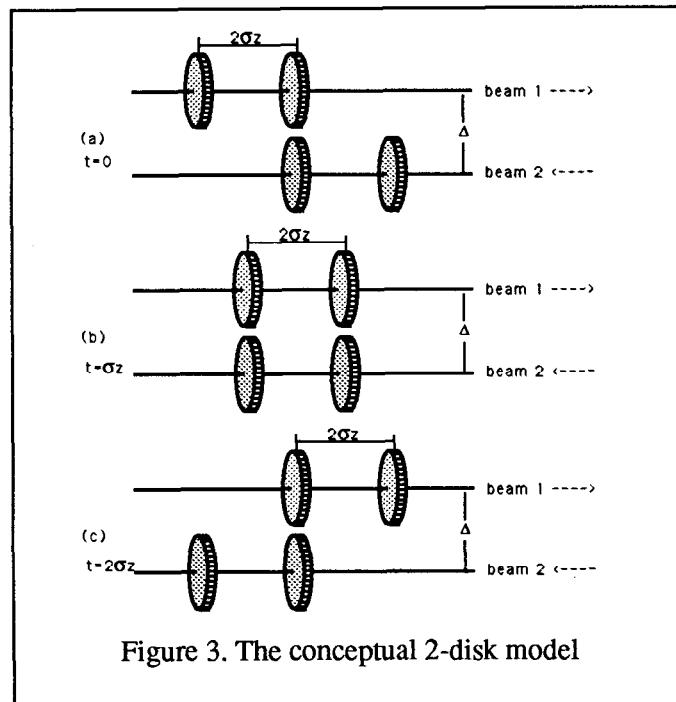
Figure 3. The conceptual 2-disk model
