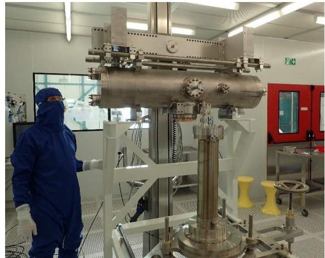
Figure 10: Assembly of accelerating unit in cleanroom at CEA-Saclay.
