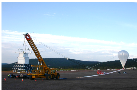
Figure 1. A picture of the HELIX payload for its first balloon flight just before launch from Esrangle, Sweden. The solar array hangs below the bottom of the white gondola.
