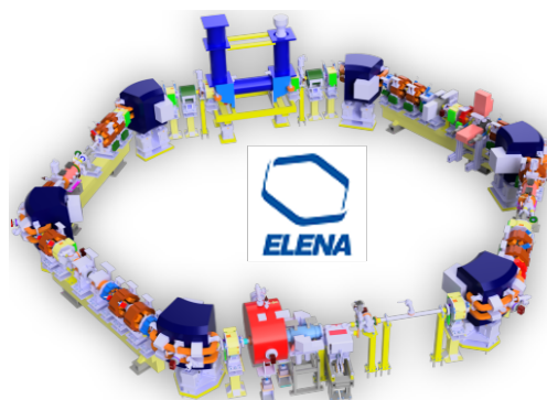
Figure 2: CAD model of the ELENA ring. The beam is travelling clockwise.
