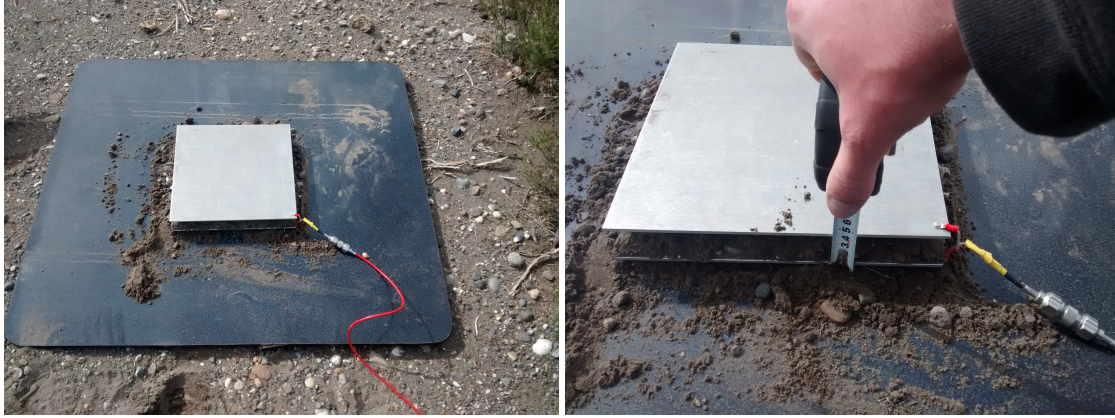
Figure 6.9: For the measurements at the AERA site, the capacitor has been placed on a wooden plate to reduce disturbing effects from the underlying soil as well as to avoid a grounding of the capacitor plates. Soil from the surface is collected and placed in between the capacitor plates. The distance between the plates is measured at multiple positions using a tapeline.
