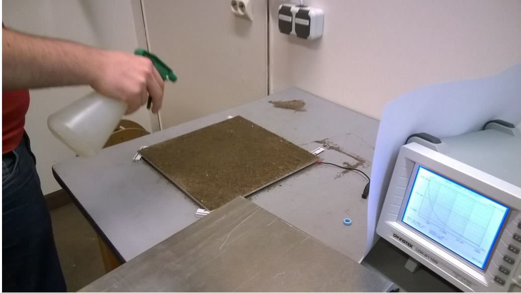
Figure 6.7: Picture of the soil sample placed in the capacitor. Different soil humidities are achieved by spraying water with different amounts of water on the soil sample.
