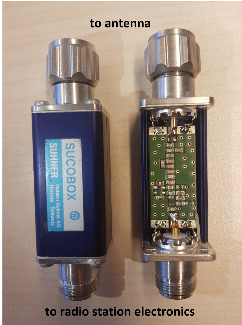
Figure 4.17: Photo of the low-noise amplifier used in the LPDA-equipped radio stations at AERA.
