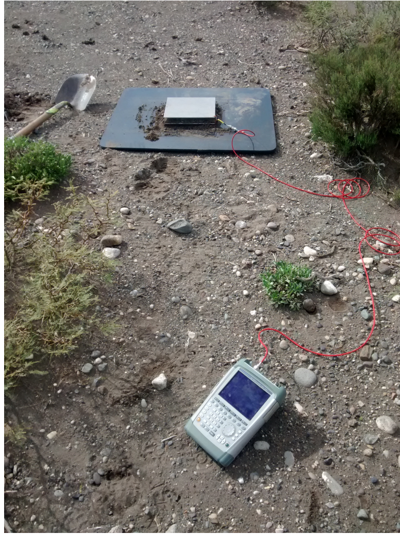
Figure 6.10: Picture of the full setup to measure the relative permittivity of soil at the AERA site using a capacitor connected to the FSH4 vector network analyzer.
