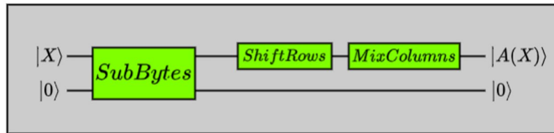
Figure 3. Quantum Circuit for A(X) .
