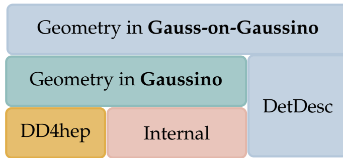
FIGURE 3.8: Dependencies of GAUSSINO and GAUSS-ON-GAUSSINO on various detector description libraries.
