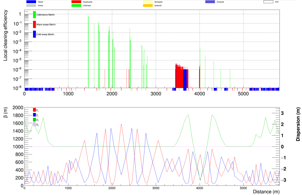
Figure 5: Loss distribution in the collimation section and lattice functions, protected superconductor magnets are used in the section
