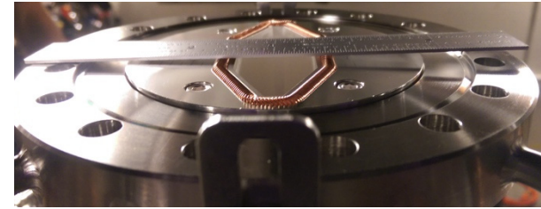
Figure 4: Flange image of the bellows with trapezoidal groove and the RF contact spring at place after disassembling.
