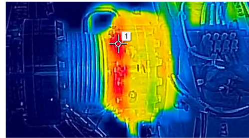
Figure 2: Thermal image of the attached bellows to the flange of the vacuum chamber made by the FLIR AX8 infrared camera, where the local overheating appeared.
