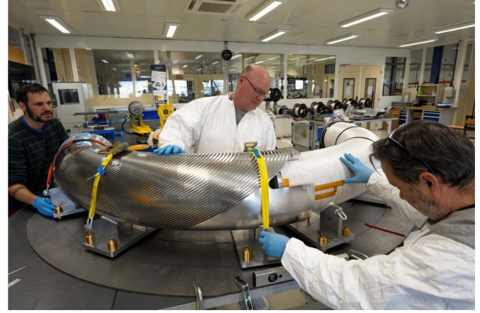
Fig. 4. Slowly sliding the outer former over the inner former.
