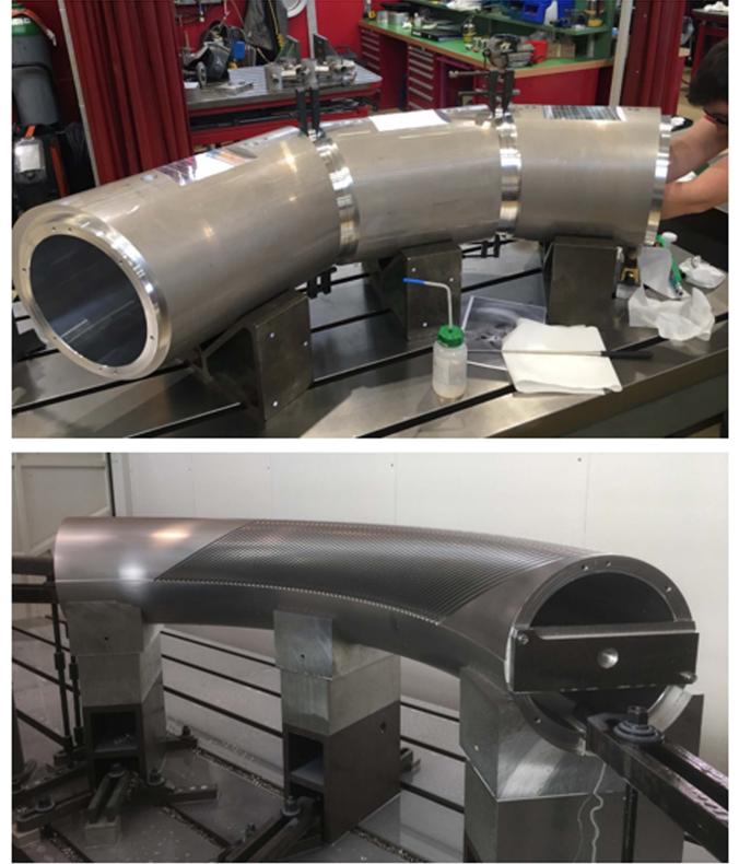
Fig. 2. Assembly of the 3 segments for the inner former, preparing for injection (top). Completed machining of the top outer surface of the assembled former (bottom).
