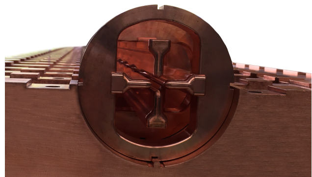
Figure 2: Electrodes mounted into the carrier-rings on the lower half-ladder structure.
