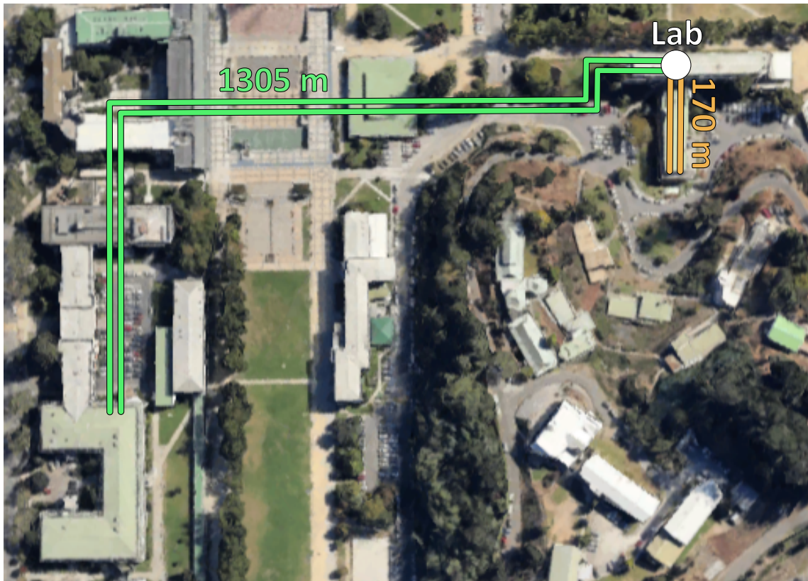
Figure 3.3.2: Map of installed fibers at the University of Concepción’s campus at Concepción, Chile. Orange lines indicate the 6 th floor channel. Green lines indicate the Faculty of Engineering channel. Numbers indicate the total path length including return paths. Vertical sections of fiber from the laboratory to the 6 th floor and Faculty of Engineering buildings not shown.
