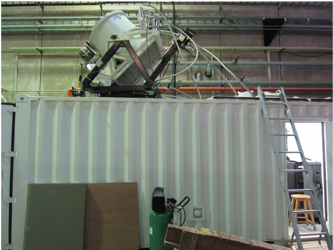
Figure 5.3: Photograph of the ABS experiment from the side. The base and receiver are raised to the roof as they will be for observations in Chile.
