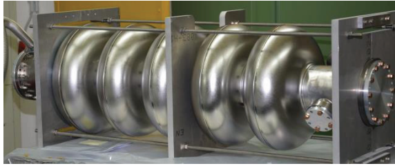
Figure 1: ESS high beta prototype cavity n°1 (up) and n°2 (down) at factory before shipment.
