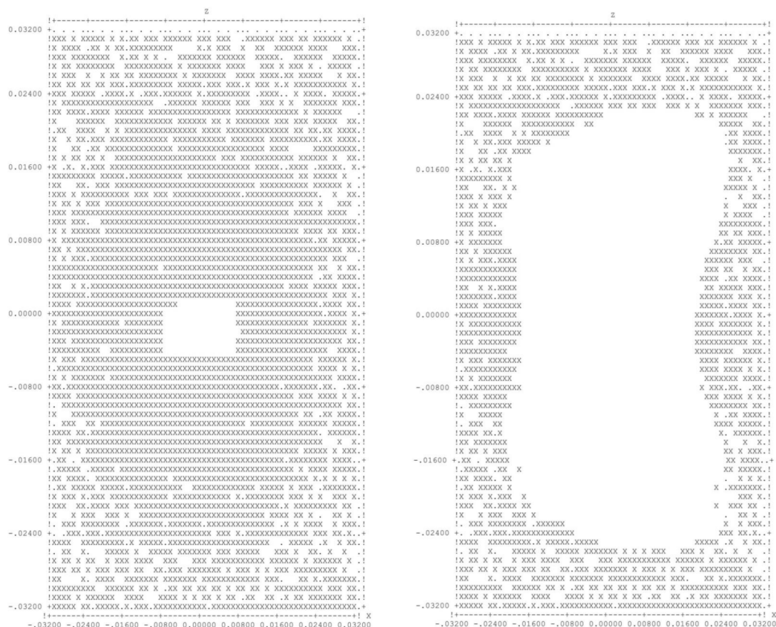
Figure 4: Dynamic apertures of the NESTOR (left) and storage ring with RF harmonics number h = 36 .
