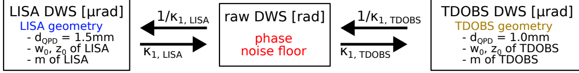
Figure 5.3: Scheme of the comparison principle between LISA's DWS measurements and TDOBS's DWS measurements.
