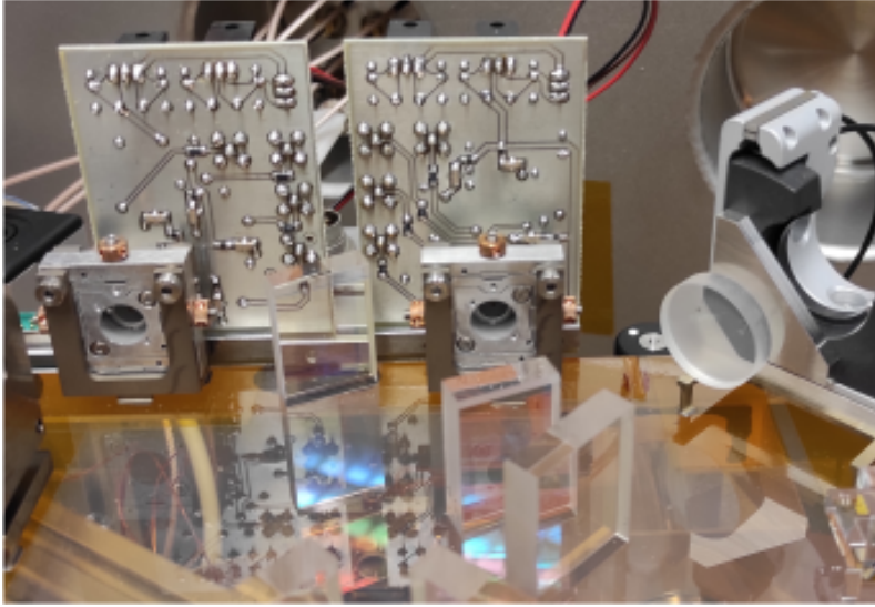
Figure 3.16: Photo of the REFQPD1 and REFQPD2 PDs featuring TIA #2, mounted on the flexure mounts and with the TIA PCBs attached right on the back.
