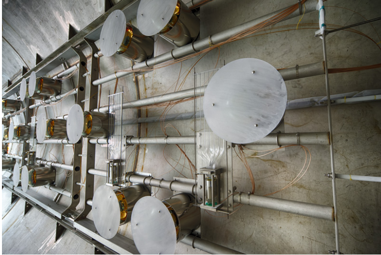
Figure 3.6.: Photograph of the PMT array mounted on the inner cryostat wall before the TPC was installed. A group of six PMTs is arranged in a circular array. The flat wavelength-shifting TPB plates are placed in front of them. From Ref. [32].
