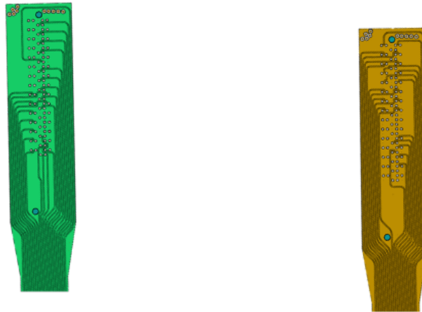
Figure 42: Picture of the data differential pairs in the Type-0 to PP0 flex at the PP0 connector. This area is the most significant constraint in designing the PCB. All data was still able to be routed on two layers.
