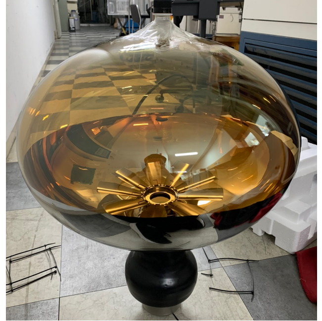
Fig. 3. (Color online) 20-inch MCP-PMT : The photocathode of orange color is the transmission photocathode, which is coated on the inner surface of the glass. The reflection photocathode is the silver-coated inside of the glass. MCP is the circular structure in the PMT center. The experimental structure was attached on the top of the PMT.
