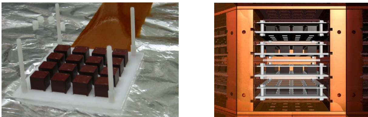
Figure 1. A photograph of the first layer of the 64-crystal proto-type (left) and an artistic impression of the whole array in the copper mounting structure (right).
