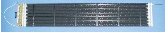
Figure 2-9: A 0.6 m long space-qualification TRD module of 16 proportional tubes.
