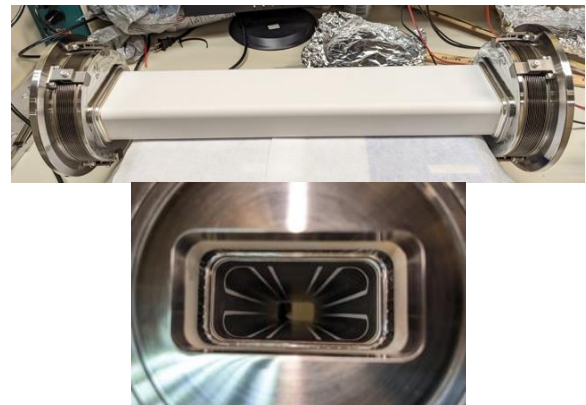
Figure 3: PAR kicker chamber with patterned Ti coating.
