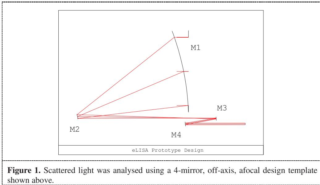
**Figure 1.** Scattered light was analysed using a 4-mirror, off-axis, afocal design template shown above.
