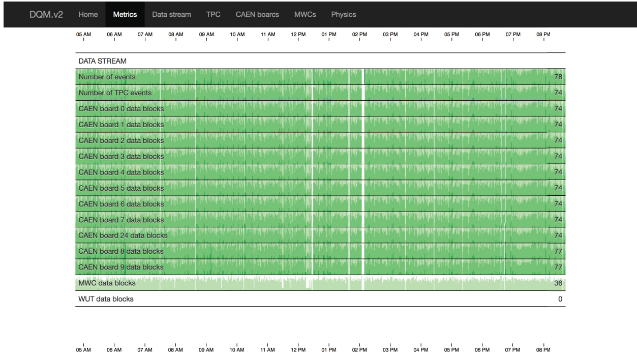
Figure 3.17: DQM monitoring page displaying a set of time series plots of the number of data fragments collected per super cycle over the previous 16 hours of operation.
