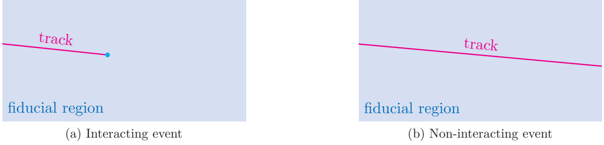
Figure 5.9: The interacting length is defined to be the length of a reconstructed track within the fiducial region up to the interaction point of an interacting event. The non-interacting length is defined to be the length of a reconstructed track within the fiducial region of a non-interacting event.
